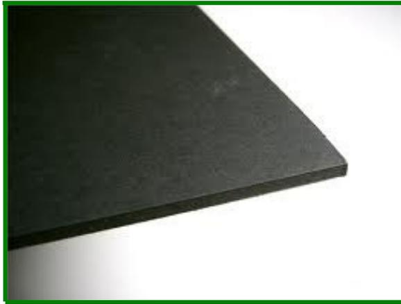
The substrate is closed cell expanded rubber with a thickness of 3.94 mm.
