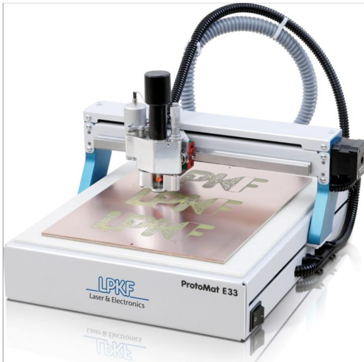
A CNC **milling machine** is used to pattern the conductive surface and to drill the holes in the paper.
