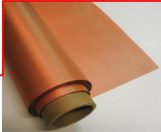
The metal layers are an electrotextile called **Flectron<sup>®</sup>**.
