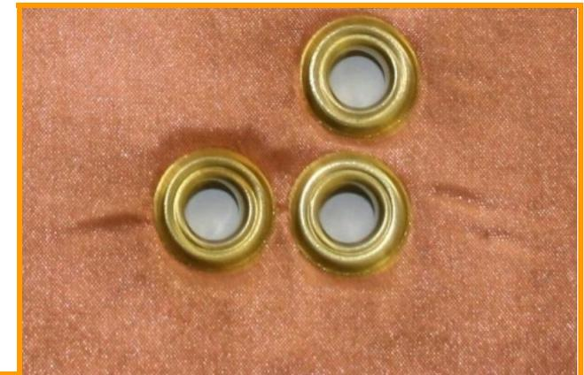
**Rivets** are used for the metallization of via holes
