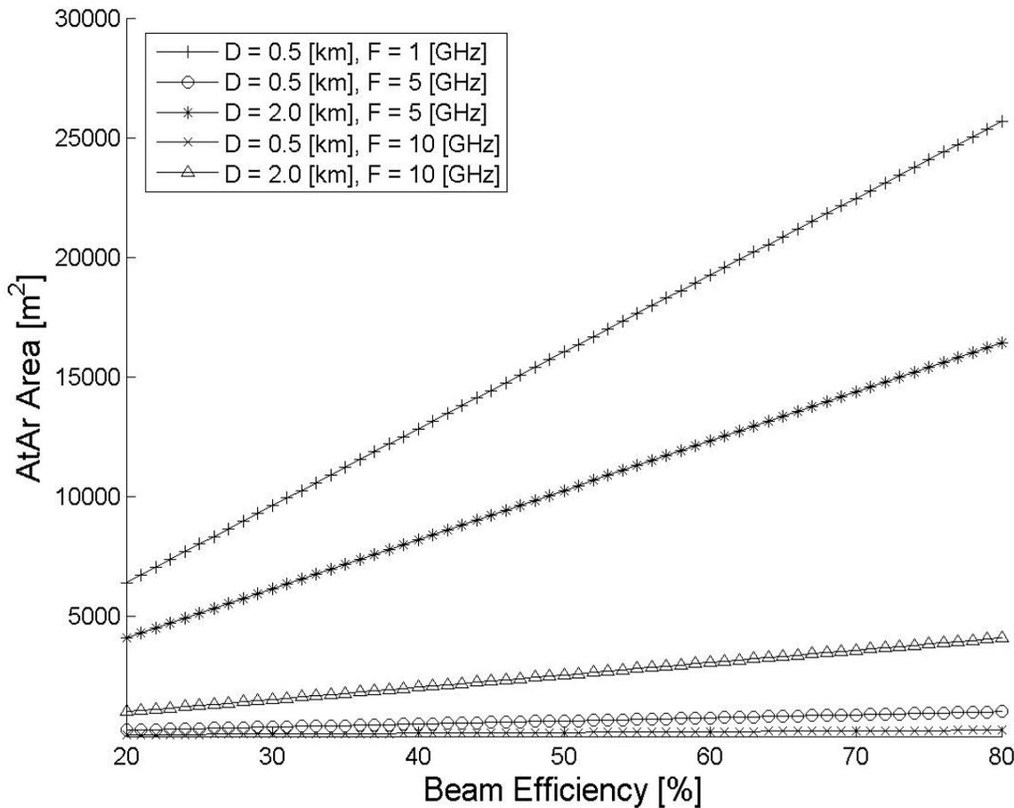
Example plot of product of transmit and receive apertures, in square meters, for 3 frequencies and 2 ranges (R=D=0.5 and 2km). The graph shows how the size varies as a function of beaming efficiency.
