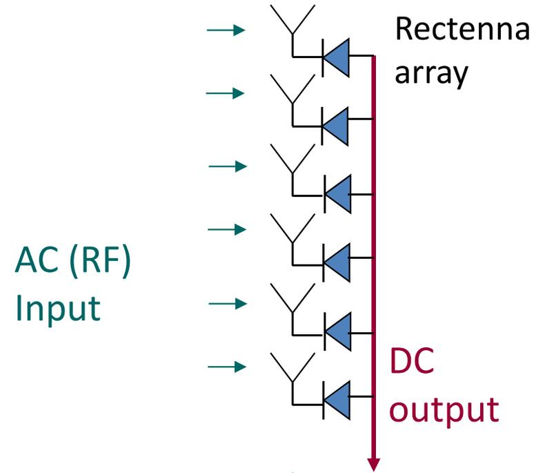
Array of antennas integrated with rectifiers
