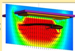
Fig. 4 Magnetic field representation between coupled coils
