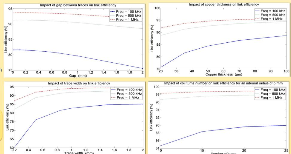
Fig. 5: Coil parametric study on Gap (top left), copper thickness (top right), trace width (bottom left) & turns number with Rin=5mm (bottom right). All parameters except the analyzed one were constant and identical to basis coil's ones.
