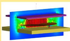
The maximum link efficiency is obtained for  $d=2\text{mm}$ ,  $\mu_r > 100$  and  $\text{RAR} > 1$ . By using a ferrite the link efficiency was improved with 4% at 100kHz.
