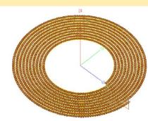
Fig. 3 Basis coil (N=10, Rin=10mm, Th<sub>Cu</sub>=35µm, wt=0.8mm & Gap=0.2mm)
