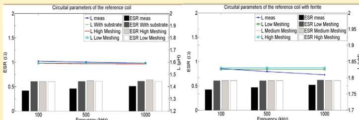
Fig. 2 shows there is no need to include the FR-4 dielectric in the model or to use high meshing densities at chosen frequencies.
